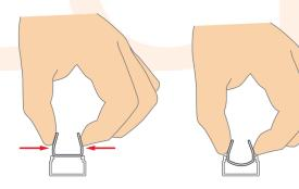
When inserting U-Clip 30 in 25x16mm trunkings, gently squeezing the upright tabs causes the base to compress for tight fitment in Size 2 trunkings.
